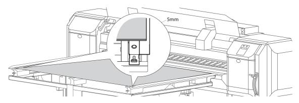
[7] From the rear side of the printer, insert the rigid media into Media feed slot.
