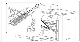
Use a dropper to moisten the cleaning wiper with maintenance cleaner.
