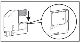
Slide the S/C card into the tabs of the adapter.
