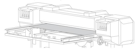
[8] If the right edge of the roll media goes further right from the loading mark when seen from the front, adjust the position of Media-feed table's rails.
