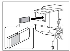
Insert cleaning cartridges into Ink cartridge slots.
