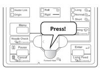
Press down the [-] key on Operation panel for a while, and check that the rigid media can be fed no problem.
