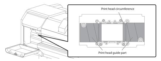
[2] Use the cleaning stick to remove the ink deposits or dust on the bottom of the carriage.
