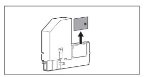
Remove the S/C card from the High capacity ink pack adapter.
