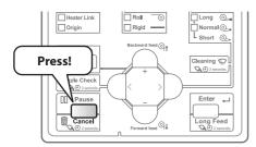
Press and hold the operation key on the operation panel for two seconds or more during printing.
