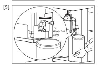
Open the waste fluid valve, and transfer the waste fluid to the container.
