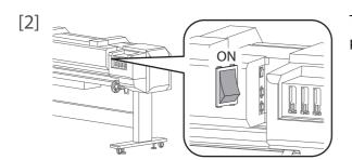
Turn ON the power switch of blower heater on the rear side of the printer.
