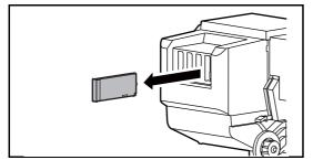
Wear the plastic gloves, and then remove ink cartridges from Ink cartridge slots.
