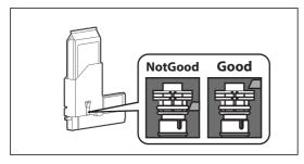
Confirm ink bag is fully seated by checking the lock mechanism is at the top of the ink delivery neck through the observation window, see proper placement in illustration left.
