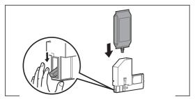
Lower the lock lever on the High capacity ink pack adapter and insert the ink bag.
