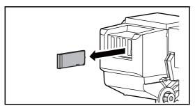
Remove ink cartridges from Ink cartridge slots.
