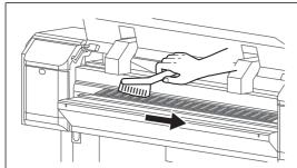
Brush off dusts on the pressurizing rollers with a soft brush.
