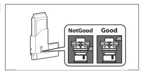
Confirm that the ink bag is inserted all the way and is locked.
