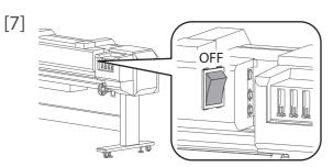
Turn OFF the power switch of Blower heater.
