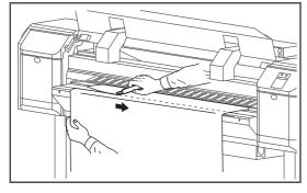
Place a razor blade on the media cut groove on the media guide, and cut the roll media.
