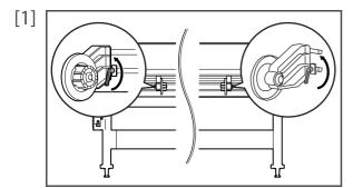
Loosen Fixing levers on the Roll media holders (both left and right) on the back of the printer.
