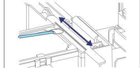
Clean off the ink on the left edge of the part, located between the flushing box and cleaning wiper.
