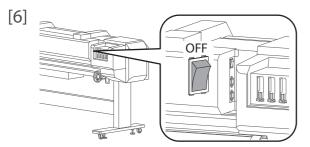
Turn OFF the power switch of Blower heater.
