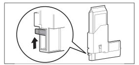
Make sure that the lock lever of the High capacity ink pack adapter is back to its original position.
