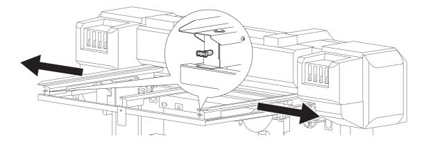
[5] Place the rigid media on the rails and tighten the rail retaining screw at where there is a 5 mm gap between the stoppers on both sides and the media.
