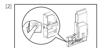
Using the paper towel provided with the printer to wipe off the ink attached to the insertion point for High capacity ink pack adapters.
