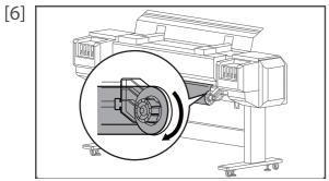
Rewind the roll media a little by rolling Flange on Roll media holder while holding the edge of the media, and eliminate any slack or slant.
