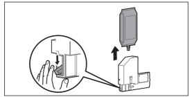
Lower the lock lever on the High capacity ink pack adapter and detach the empty ink bag.
