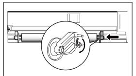
Attach Roll media holder (right) to the roll media and tighten Fixing lever.
