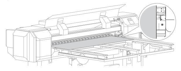
[9] If needed, use a slide lock lever on the pressure rollers to individually cancel the holddown pressure.
