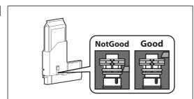
Confirm that the cleaning bag is inserted all the way and is locked.
