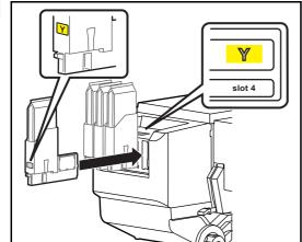
Re-insert the High capacity ink pack adapters into Ink cartridge slots.
