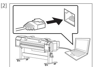
Connect the Ethernet cable to the computer.
