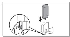
Lower the lock lever on the High capacity ink pack adapter and insert the cleaning bag.
