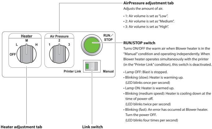
Adjusts the heater temperature.
