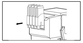
Wear the plastic gloves, and then remove High capacity ink pack adapters from the ink cartridge slots.
