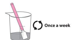
Prepare another cleaning stick to clean the cleaning wiper and around the capping unit.
