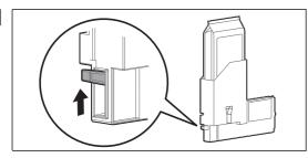
Confirm that the lock lever on the High capacity ink pack adapter is in its original position.
