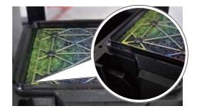
Use the dropper to moisten the absorber of the capping unit with maintenance cleaner.
