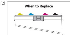
Check the absorption material for the flushing box.
