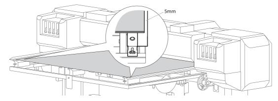
[6] Place the rigid media on Media-feed table (front side) in the same way, and fix the rails at where there is a 5 mm gap between the stoppers on both sides and the media.
