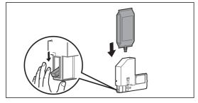
While lowering the lock lever of the High capacity ink pack adapter, insert an ink bag.
