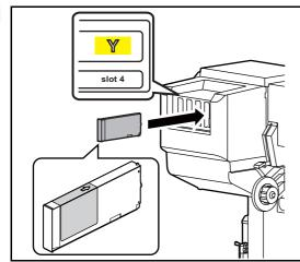
Insert new ink cartridges into Ink cartridge slots.
