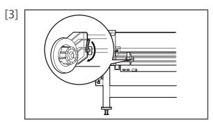
Tighten Fixing lever of Roll media holder (left) and fix the Roll media holder (left).
