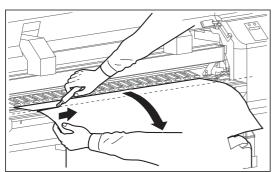
Pull the media towards you, and cut the torn part with cutting tools such as a razor blade.
