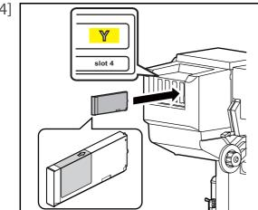
Insert new ink cartridges into Ink cartridge slots.
