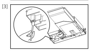
Tilt High capacity ink pack adapters, use cleaning stick provided with the printer, and absorb the ink collected around the tube connectors.
