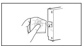
Using the paper towel provided with the printer to wipe off the ink attached to the printer plug of lnk cartridge.
