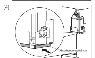
Press on the absorbent material tray of the waste fluid valve to store it.
