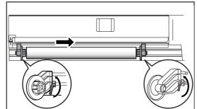
Loosen the Fixing levers of the right and left Roll media holders, move the roll media to the center.
